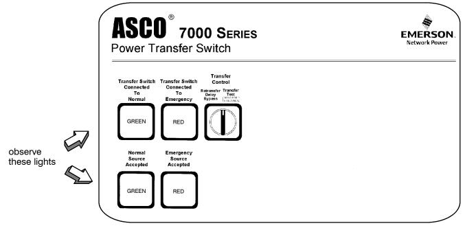
Figure 1-4. Standard controls and indicators.
